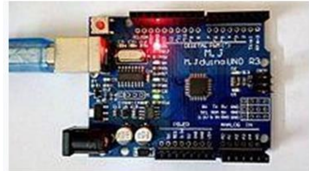
power led (red) and user led (green) attached to pin 13 on an arduino compatible board
