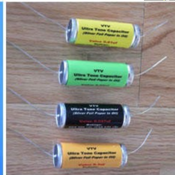
Oil-impregnated paper capacitor
