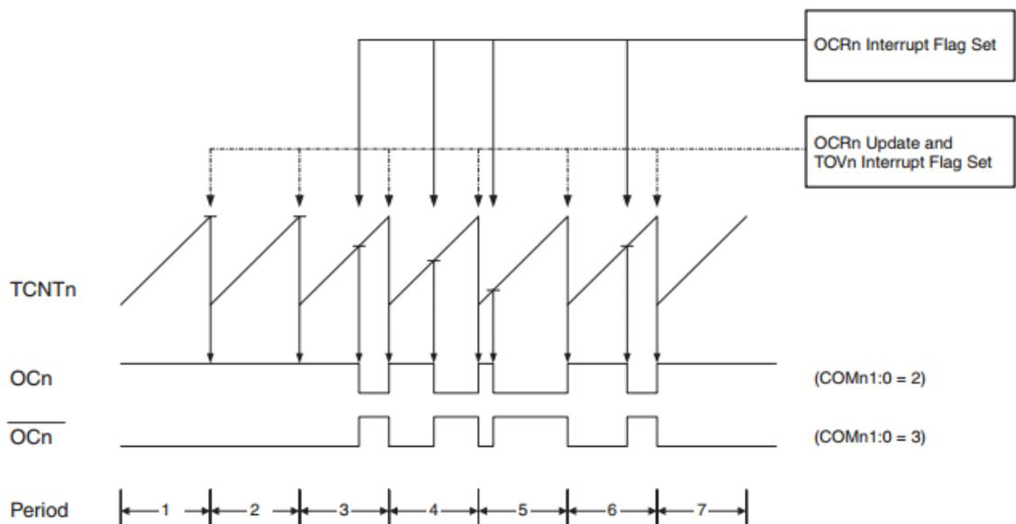
In the above picture, Compare Output mode (COMx1:0) is set in such a way that the OCx gets set whenever an overflow occurs, and to clear the OCx pin whenever an output compare match occurs (i.e. COMx1:0 = 2). The same timing diagram in the case of Timer 1 is shown below. Please note that the OCn and its complement shown in the figure below are wrong. You can see that in the case of Timer/Counter 1, the value till which TCNTx counts is determined by the TOP value.
