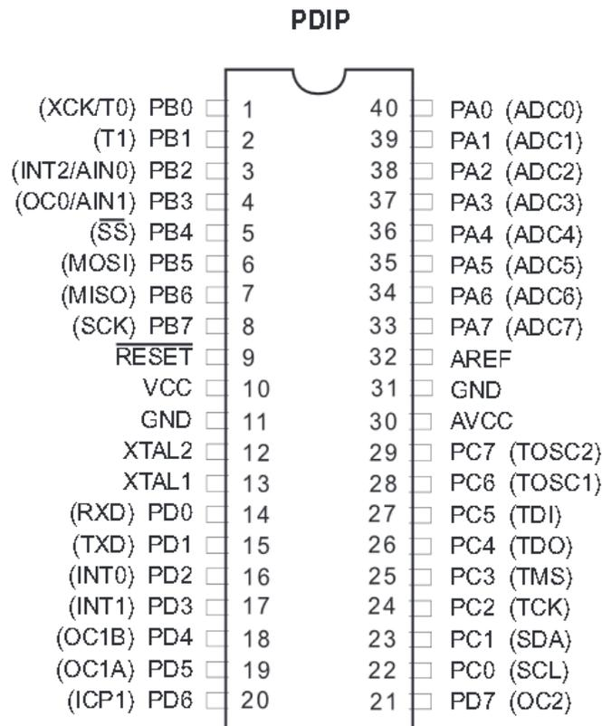
This is the pin diagram of the Dual Inline Package of ATmega 16. The microcontroller is also available in TQFP and QFN packages. Mentioned just for your information.
