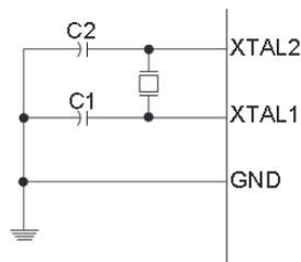
We cannot connect any arbitrarily fast crystal to the microcontroller. For the ATmega 16, the maximum crystal frequency is 16 MHz whereas it is 8 MHz for ATmega 16L.
