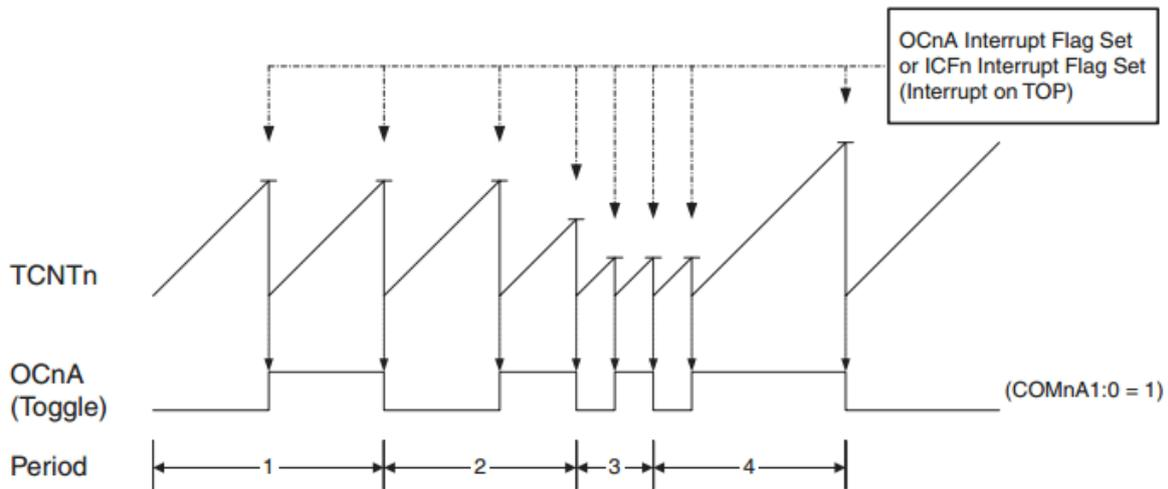
It is clear from the timing diagram that the OCx value gets toggles whenever the TCNTx value equals the OCRx value. At that instant itself the TCNTx value is reset to zero. “Oh god, are you telling me that I have to sit and find the frequency of the generated square wave? I am lazy enough to leave this job undone.” Well, no need to worry. You can find the timer output frequency using the following equation:
