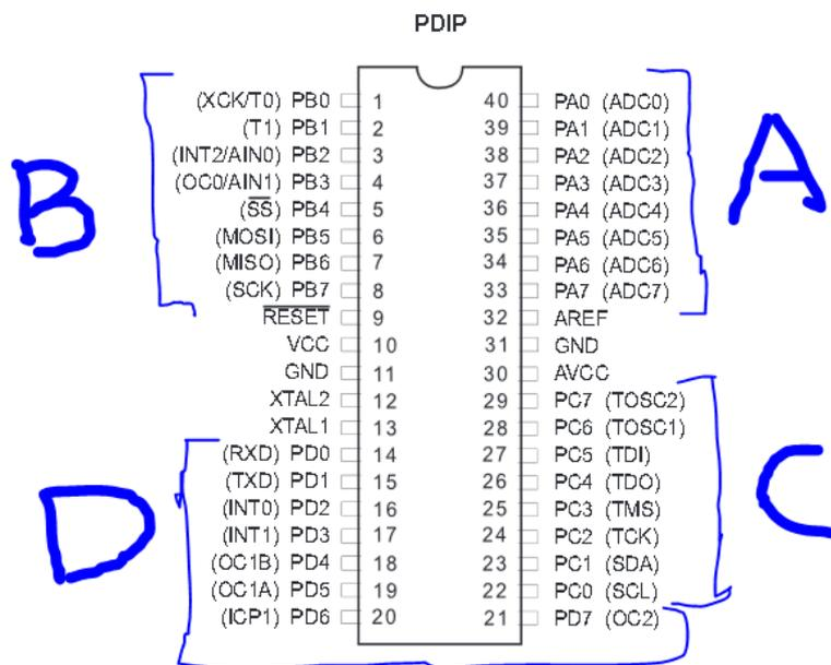
It is clear that each of these ports contains 8 pins. For example, PORTA contains pins PA0...PA7. They are clubbed into 8 because the microcontroller is 8-bit. Each port is byte addressable. We will come to that later. So in total there are 32 GPIO pins in an ATmega 16.
